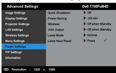
**QUICK SHUTDOWN**—Select On to turn off the projector with a single press of the Power button. This function allows the projector to quickly power off with an accelerated fan speed. Slightly higher acoustic noise is expected during quick power off.
