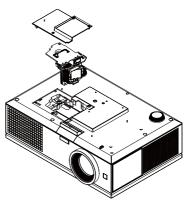
Advanced Setting menu on page 51). When a new lamp module has been changed, the projector will automatically detect and reset the lamp hours.
