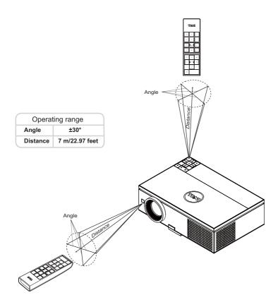
**NOTE**: Actual operating range may slightly differ from the diagram. Weak batteries will also prevent the remote control from properly operating the projector.
