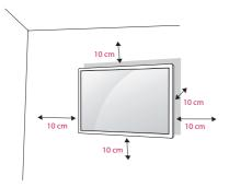
To install your monitor on a wall, attach a wall mounting bracket (optional part) to the back of the monitor.
