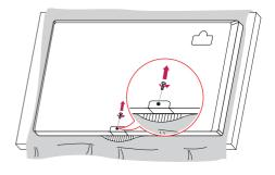
2 After removing the screw, remove the LG Logo. Attach the LG Logo Bracket with a screw, aligning it with the hole on the right side.
