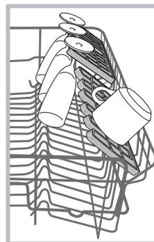
Wine glasses can be placed safely in the tip-up compartments by inserting the stem of each glass into the corresponding slot.
