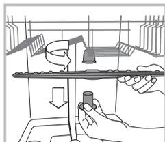
To remove the upper spray arm, turn the plastic locking ring in an anti-clockwise direction. The upper spray arm should be replaced so that the side with the greater number of holes is facing upwards.
