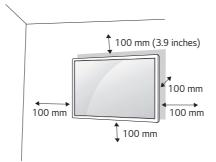
To install your monitor on a wall, attach a wall mounting bracket (optional part) to the back of the monitor.
