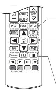
**PSM** Selects the Picture Mode. **HOME** Activates the Launcher. **W.BAL** Enters the White Balance menu.
