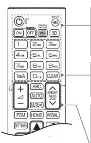
(**DOWER**) Turns the monitor on or off. **MONITOR ON** Turns the monitor on. **MONITOR OFF** Turns the monitor off. **ENERGY SAVING** Reduces power consumption by adjusting peak screen
