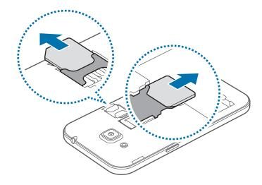
▶ Single SIM models: Press the SIM or USIM card with your finger, and then pull it out.
