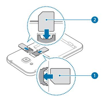
► Single SIM models: Insert the SIM or USIM card with the gold-coloured contacts facing downwards.
