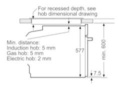
measurements in mm
