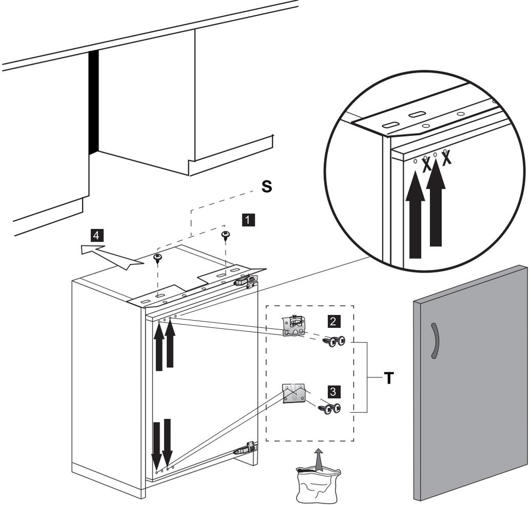
**Note:** Installation step for 2, screws for connecting top plastic part should not be screwed very hard, because of moving the plastic part easily left or right side.
