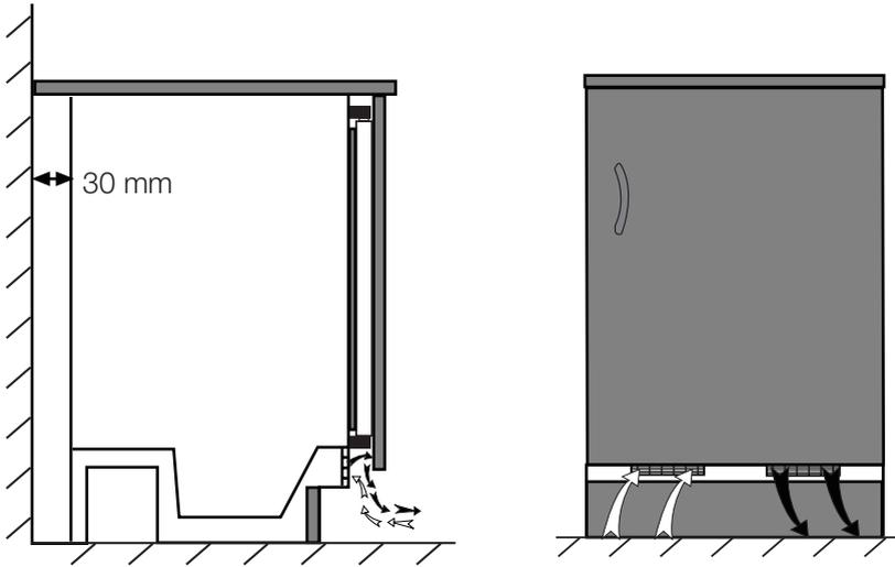
To avoid any loss in performance, air suction channels should not be obstructed. (140 cm<sup>2</sup>)
