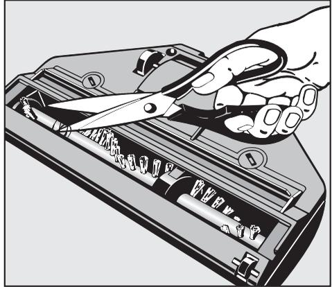
For more obstinate tangles or blockages inside the Turbobrush, the cover can be opened. Any large particles can then be easily removed.
