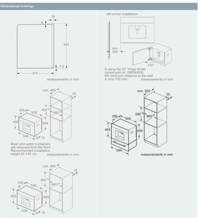
Bean and water containers are removed from the front. Recommended installation height 95-145 cm. measurements in mm
