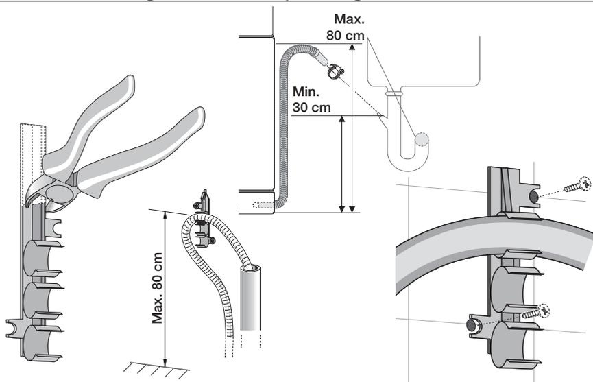
1. Remove the hose holder which is attached to the product and cut off part of the holder as shown in the figure.
