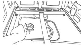
4. Disassemble the coarse filter and micro filter.
