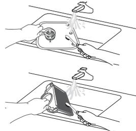
6. Reassemble the filters in the reverse order of the disassembly, replace the filter insert, and rotate clockwise to the close arrow.
