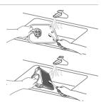
6. Reassemble the filters in the reverse order of the dissasembly, replace the filter insert, and rotate clockwise to the close arrow.
