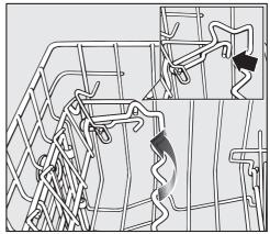
■ Pull the rail upwards and click it back into position at the required height.
