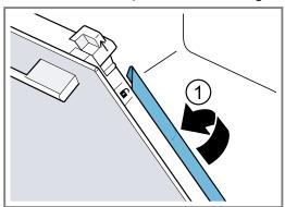
**4. Note:** The word "Pyro" must be legible on the top left of the inner pane.
