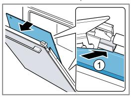
2. Note: The intermediate pane is automatically positioned by the rotational movement of the spacer. Slide the second intermediate pane into the central retainer 1 and fit it at the top.
