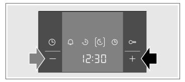
After a few seconds, the oven adopts the settings and switches to standby. The display shows the time at which the dish will be ready and the 🖔 symbol is in brackets. The symbols 🔾 and 🖰 go out. When the main oven starts, the cooking time counts down in the display and the 🖒 symbol is shown in brackets. The 🖔 symbol goes out.
