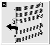
The rails fit both the left and right sides. Ensure that, as shown in figure B, levels 1 and 2 are below and levels 3, 4 and 5 are above.
