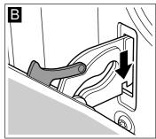
Fold back both locking levers (figure C). Close the oven door.
