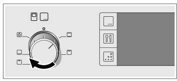
Set the temperature or grill setting using the temperature selector.
