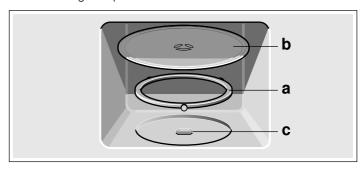
**Note:** Do not use the appliance if the turntable is not in place. Ensure that it is properly slotted into place. The turntable can turn clockwise or anti-clockwise.
