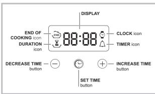
The Main Oven can be controlled by the automatic timer.
