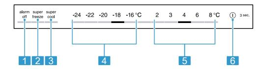
2 alarm off switches the warning signal off. super freeze switches Super freezing on or off. super cool switches Super cooling on or off. Displays the set temperature for the freezer compartment in °C. Displays the set temperature for the refrigerator compartment in °C. ① 3 sec. switches the appli-
