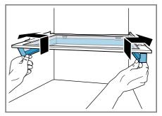
To release the rear hooks, lift up the sealing frame and slide it backwards.
