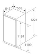
measurements in mm
