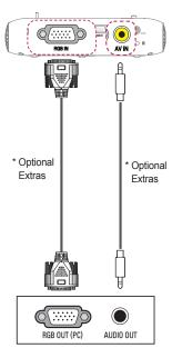
You can connect the audio cable without using a gender as shown in the illustration above.
