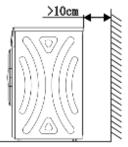
The tumble dryer will expel moist air, and it's recommended this is directed outside to avoid condensation accumulating inside a room. Position the vent hose supplied, through a window or an air outlet so that the moisture can escape. Contact a qualified tradesman to fit the vent hose so it exits through a wall or door.
