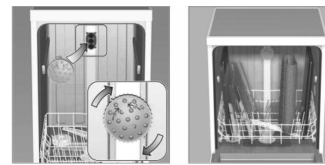
Large sheets or grilles and plates which have a diameter greater than 30 cm (gourmet plates, pasta plates, dinner plates) can be cleaned with the aid of the spray head. To do this, remove the top basket and insert the spray head as illustrated in the diagram.
