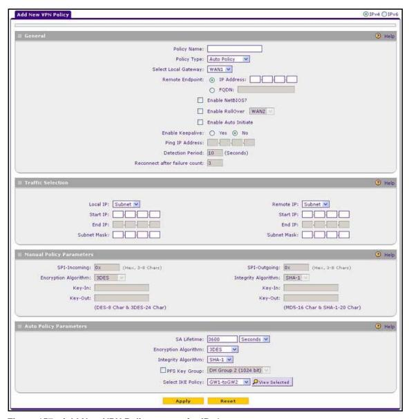
Figure 157. Add New VPN Policy screen for IPv4
