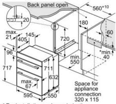
\* For installation under an induction hob, min. 50 measurements in mm
