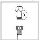
cold water tap using a 3/4 gas threaded connection (see figure). Before performing the connection, allow the water to run freely until it is perfectly clear.
