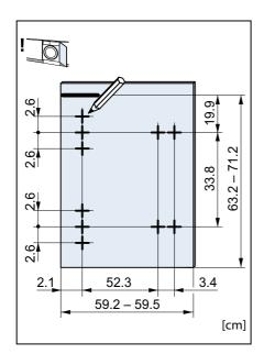
**8.** Drill the holes. Use a Forstner bit for the 35 mm hole.
