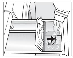
■ Add the fabric conditioner or liquid starch to the ℜ compartment or insert the appropriate capsule. Do not exceed the maximum level mark.
