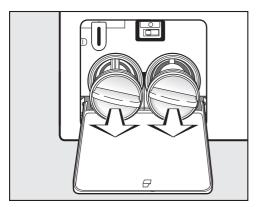
■ Remove the drain filters completely.
