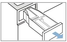
Pour a bottle of the original appliance care product and approx. 1 ½ litres of hot tap water into the condensation container.
