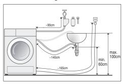
**Note:** If the hose holders are used, the possible hose lengths are reduced!
