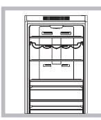
The No Frost system circulates cold air continuously to collect humidity and prevent ice and frost formation. The system maintains an optimal humidity level in the compartment, preserving the original quality of the food, preventing the food from sticking together and making defrosting a thing of the past. Do not block the aeration cells by placing food or containers in direct contact with the refrigerating back panel. Close bottles and wrap food tightly.
