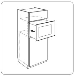
4. Open the door and fix the appliance to the cabinet with a screw.
