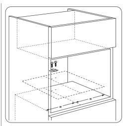
3. Install the appliance. Make sure the bracket locks the back of the appliance.
