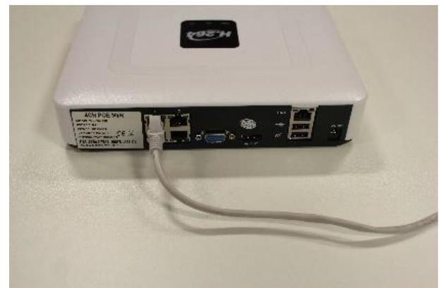
Insert the plug provided into the mains power socket. After this attach the cable to the power port in the back of the NVR (as shown in diagram 1). This will give power to the NVR and a light will appear on the front of the unit.
