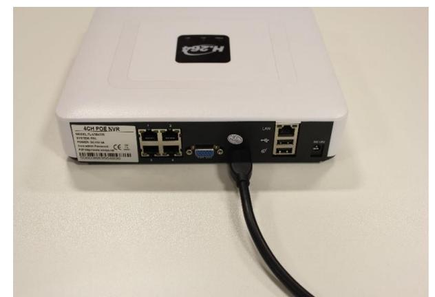
If you wish to connect your NVR to the internet so you can view the footage remotely you will need to use an Ethernet cable. Insert one end of the Ethernet cable into the Ethernet port on the back of the NVR (as shown in the image to the right) and then insert the opposite end of the cable into your internet router.
