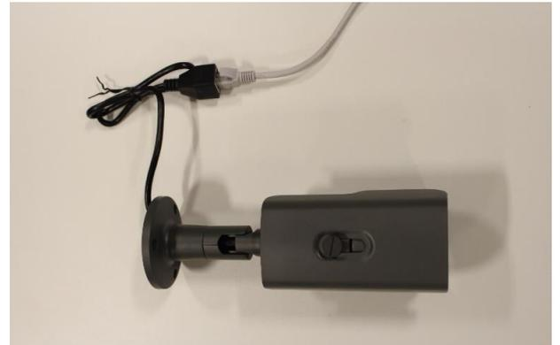
Plug the cables attached to the cameras into channels 1 to 4 of the NVR. (as shown in diagram 1)
