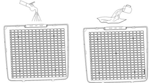
Remove the ABS filter frame. If the mesh filter is dirty, Hoover it. If it is heavily soiled wash it with warm soapy water and dry thoroughly before reinserting it in the unit.
