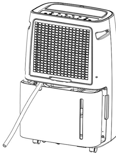
Make sure the connection between pipe and the drain outlet is tight and does not leak. Then direct the pipe to a suitable drainage point. This unit uses gravity to dispose of water hence the drain should be lower than the water outlet on the unit. Put the tank back into the unit. Be sure to run the water pipe downward and let the water to flow out smoothly. Do not kink or bend the pipe.
