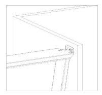
3. Hang the cooker hood on the screws between the two cupboards.
