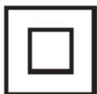
This equipment is a Class II or double insulated electrical appliance. It does not require a grounded connection.
