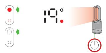
Press the red thermostat control button until the digital display shows the target room temperature. The power button light will change from blue to red to indicate that you have entered heating mode. The red circle will disappear when the target room temperature is reached. Once the target room temperature has been reached, the machine will stop heating the air. If the room temperature falls below the target room temperature, the machine will start to heat again.
