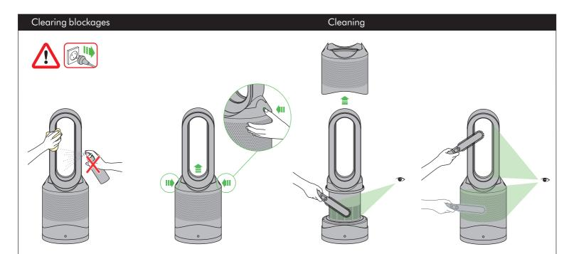
Unplug from the mains electricity supply. If the machine has been in use, leave for 1 to 2 hours before cleaning to allow the machine to cool completely. Dust may accumulate on the surface of the machine. Wipe dust from the loop, filter unit and other parts with a dry or damp cloth when dust accumulates. Do not use detergents or polishes.
