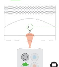
When you have reassembled your machine, press and hold the Standby on/off button for 6 seconds on the remote control to reset the filter indicator.
