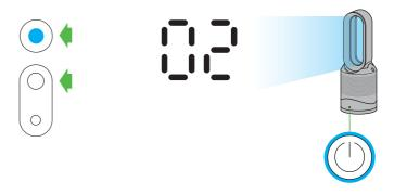
Press the blue cool mode button to enter cool mode. The power button light will change from red to blue to indicate that you have entered cool mode. To adjust the airflow speed use the airflow control button.
