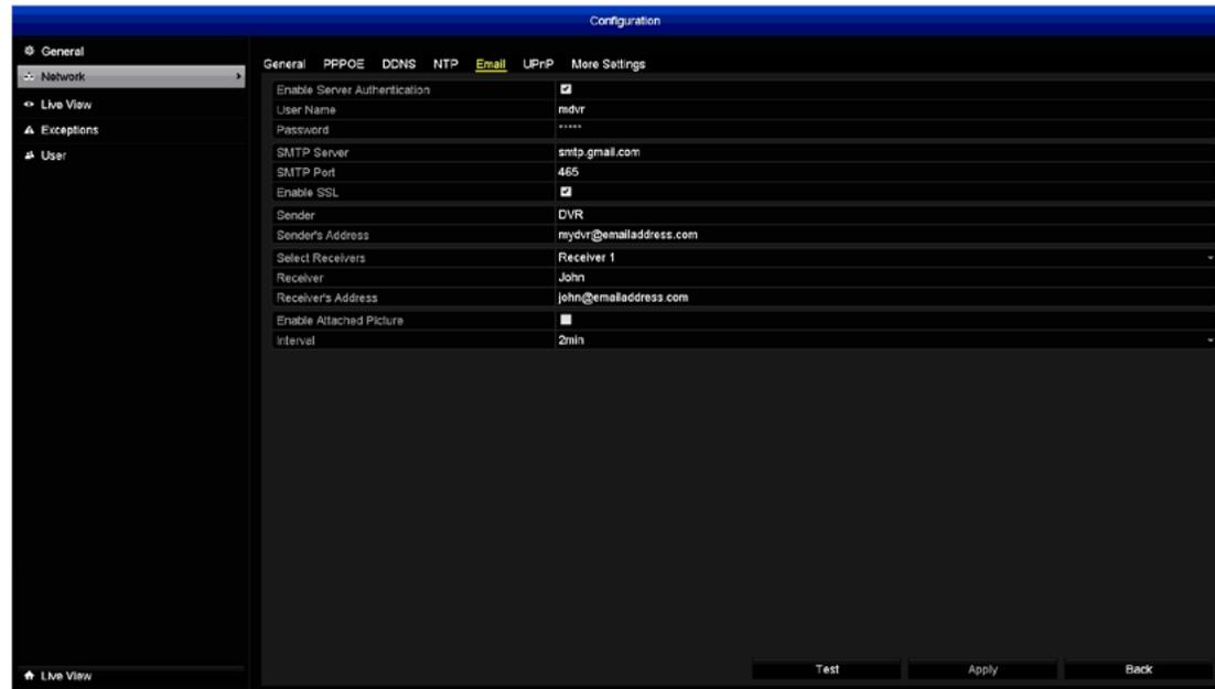
**Enable Attached Picture:** When enabled, the DVR will attach three small images when sending an email, each time there is an Event alert such as Motion Detection.
