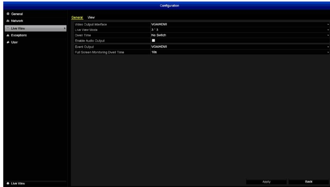
**Video Output Interface:** As the DVR has a VGA and HDMI output, this cannot be changed.
