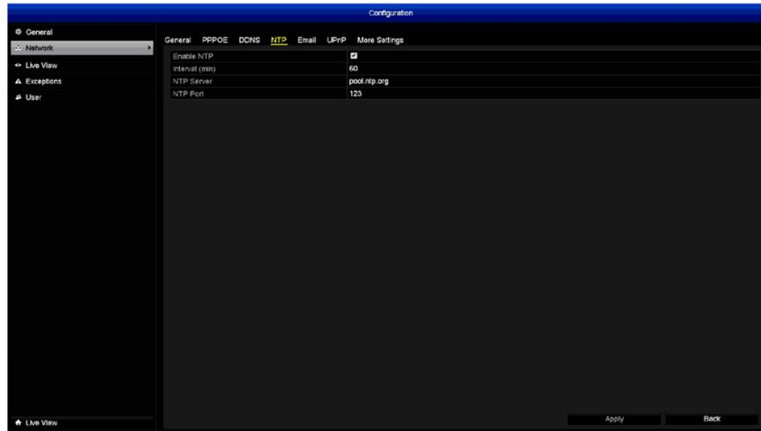
The NTP (Network Time Protocol) function allows the DVR to automatically sync its clock with an on-line server and gives it the ability to constantly have an accurate time setting. Obviously this is very important for a security system and is enabled by default. We don't recommend changing any of the default settings.
