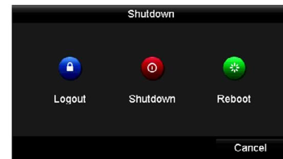
To shutdown or reboot the DVR, or simply log out of the current user account, click the "Shutdown" button. To ensure the integrity of your data and recordings, always select "Shutdown" when powering off the DVR.
