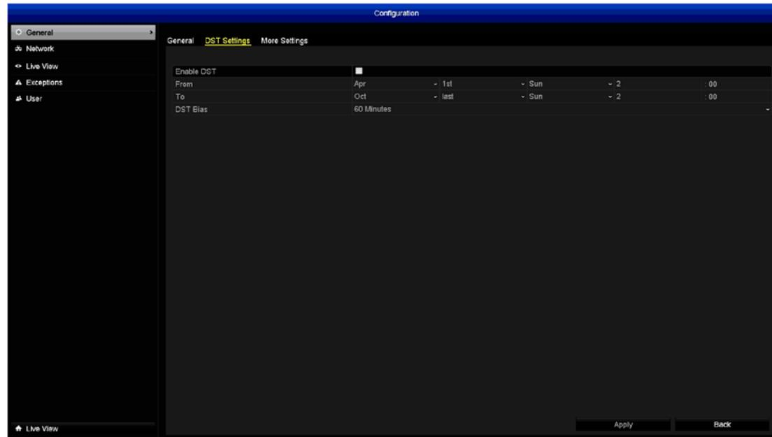
**Enable DST (check box):** Enable this setting if you would like the DVR to adjust the time when Daylight Saving begins.
