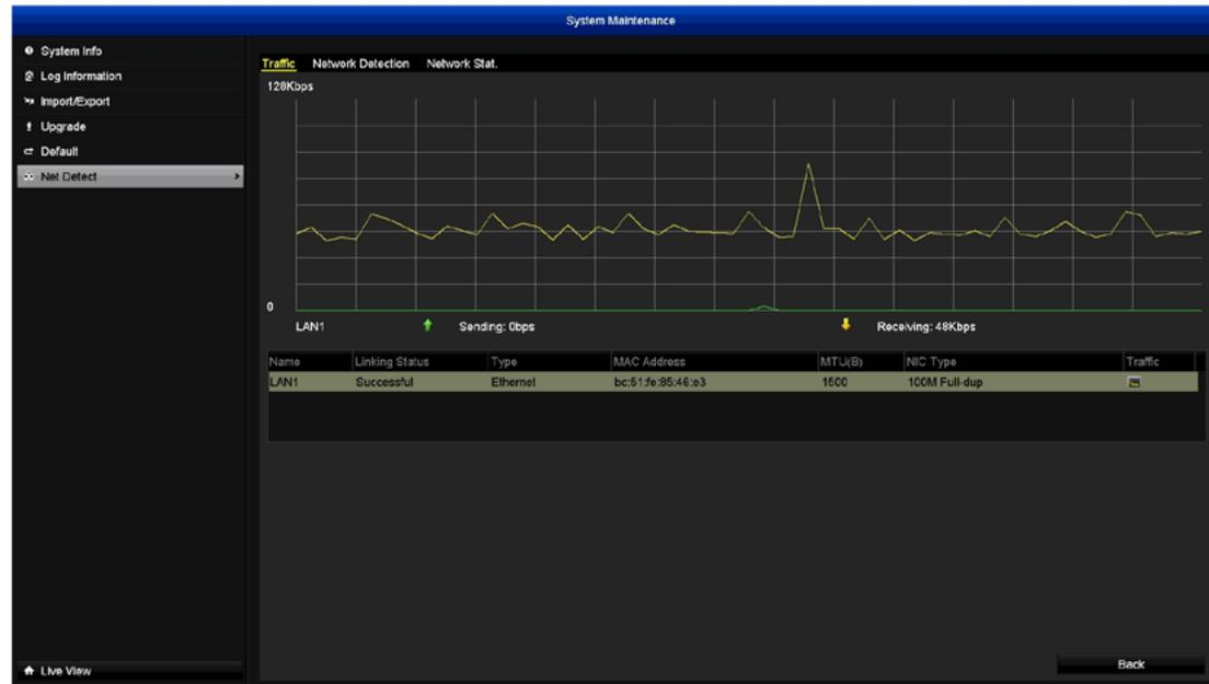
The Net Detect function allows you to check network traffic and to obtain real-time information from the DVR such as network detection, network status and sending and receiving network traffic.
