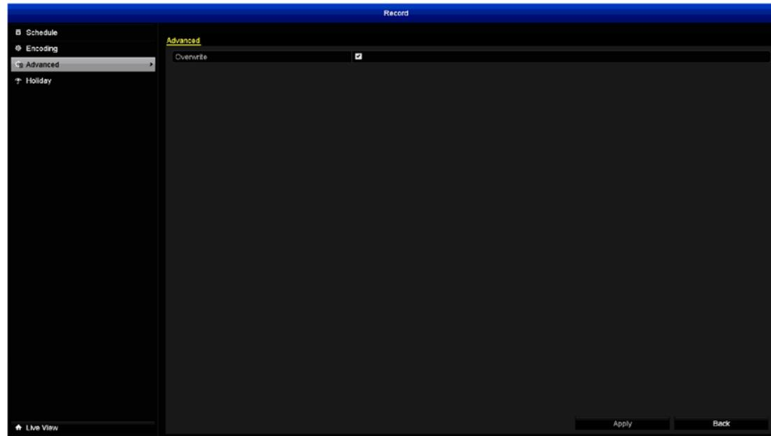
With the Overwrite function enabled, the DVR will record over previously saved files stored on the hard drive. The DVR will always record over the oldest files on your hard drive first.
