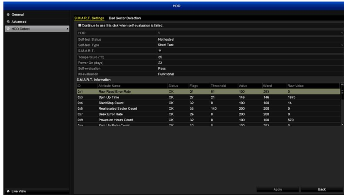
The HDD Detect function displays technical information of the hard drive installed as well as the ability to detect bad sectors.
