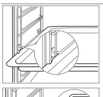
The deep pan and the wire shelf have side edges. These edges and the shape of the guide-bars are a special device to prevent the cookware from slipping.
