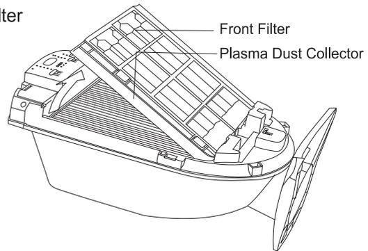
2. Lift up the tab at the top of the plastic housing for the metal dust collector grid. Once this tab is open, remove the dust collector. Please wear protective gloves to avoid any cuts on your fingers.
