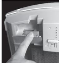
2. Take out the dust sensor and carefully unplug its connecting cord. Make note of how it is plugged in.
