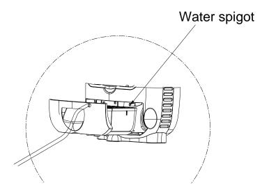
When you no longer wish to use the permanent water drainage, disconnect the drainage tube from the device. Ensure that the water container is positioned correctly.
