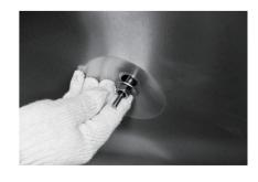
**34**Fit the Thermometer in Position using the attached Nut and Washer (H).
