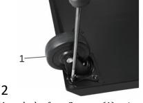
Attach the four Castors (1) using 4 Bolts (A) for each Castor.
