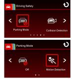
Detection, or touch screen to power off." will be displayed on the screen. This means the system will enter Motion Detection automatically in 10 seconds, when the device detects any motion in front of lens. Video Record will be activated for a duration the same as the length setting. If the screen is touched anywhere in 10 seconds, the device will be powered off instead of entering Motion Detection mode.
