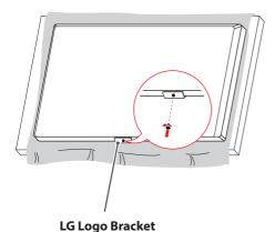
2 After removing the screw, remove the LG Logo. When re-attaching the LG Logo, repeat the process in reverse order.
