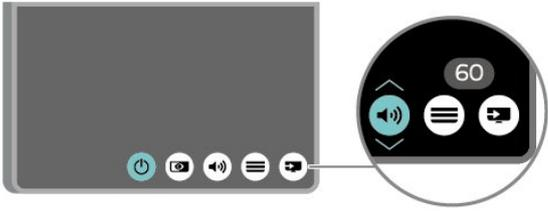
3 - Press up or down to adjust the volume or tune to the next or previous channel. Press up or down to go through the list of sources, including the tuner selection.
