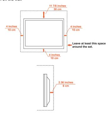
For use only with UL Listed Wall Mount Bracket with minimum weight/load: Please refer to the Specification on page 30.
