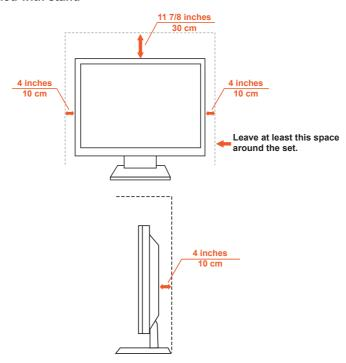
Never install the display set where air-circulation is blocked.
