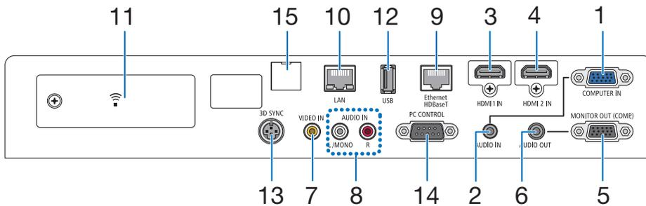
1. **COMPUTER IN/ Component Input Terminal (Mini D-Sub 15 Pin)**
