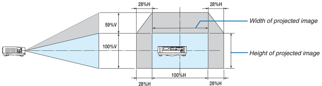
\* The lens shift range is the same for ceiling installation.
