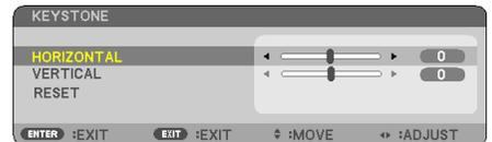
2. Press the ▼ button to select [VERTICAL] and then use the ◀ or ▶ so that the left and right sides of the projected image are parallel.
