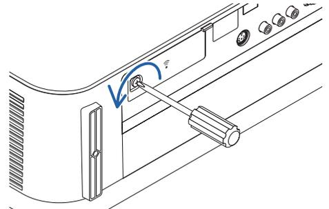
(2) Hold the head of the screw and remove.
