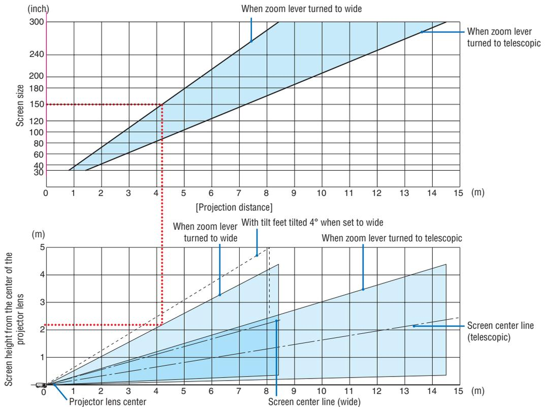
\* The figures indicated for "height of screen from projector lens center" on the projection distance table are for a lens shift of 59% V.
