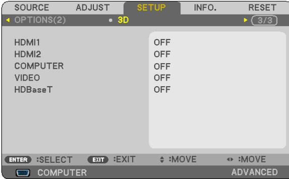
4. Press the  $\nabla$  button to select a signal and press the ENTER button.
