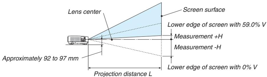
(Note) Height from lens center to lower edge of screen (with tilt feet screwed in)
