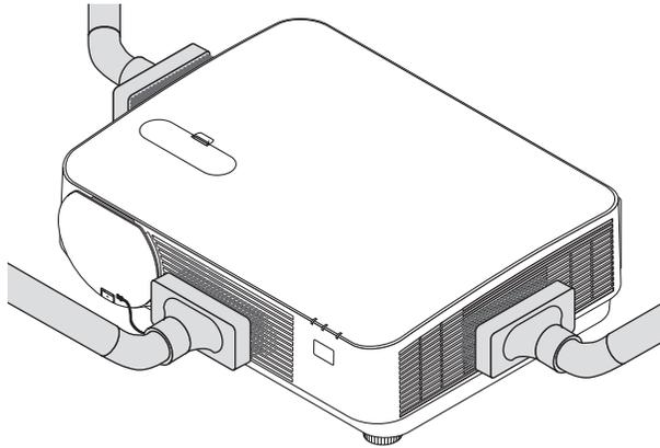
*Vacuum the dust off the ventilation slits or the speaker.*
