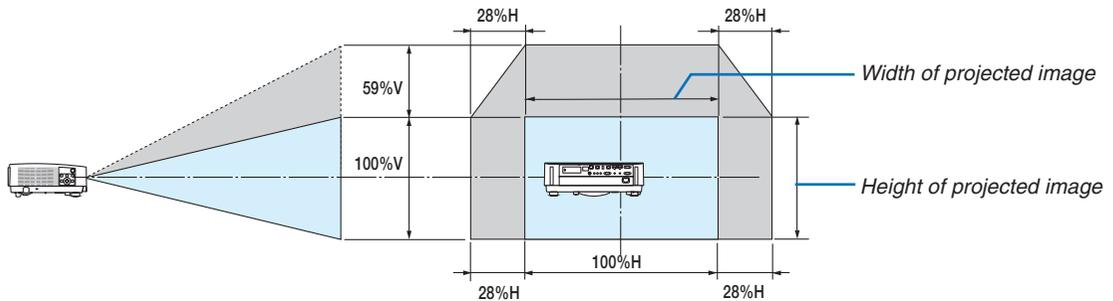
Description of symbols: V indicates vertical (height of the projected image), H indicates horizontal (width of the projected image).
