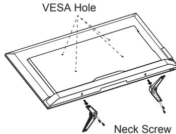
1. Loosen the screws on the button of the base, and remove the base.
