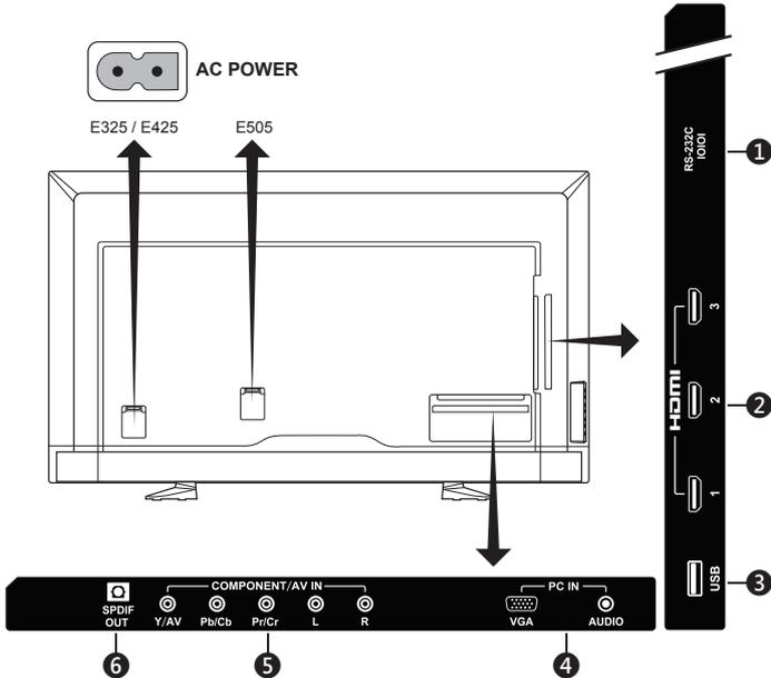
1. **RS-232C** – Connect to your PC, and receive the control commands from the PC.
