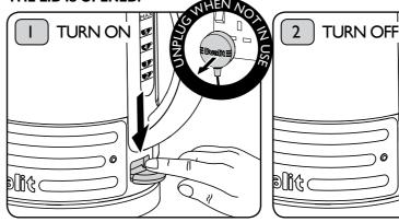
Plug the kettle into the power socket. Press the 'On/Off' switch down. The power neon will illuminate and the kettle will start to heat up. If the kettle is accidentally switched on with no water inside, the boil-dry device will switch off the heating element to prevent damage to the kettle.
