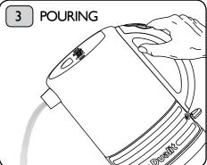
Remove kettle from the power base. When filling or carrying the kettle, do not tilt it backwards, as this may allow water to pass through the steam tube onto the control area. Should this happen, the kettle must be allowed to dry before re-using. To avoid the risk of splashing, once the kettle has boiled wait 10 seconds then pour slowly. Do not over-tilt the kettle.
