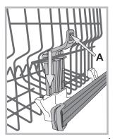
If the rack is equipped with a **Lift-Up device**\* (see figure), lift it up by holding its sides. To restore the lower position, press the levers (**A**) at the sides of the rack and follow the rack down.
